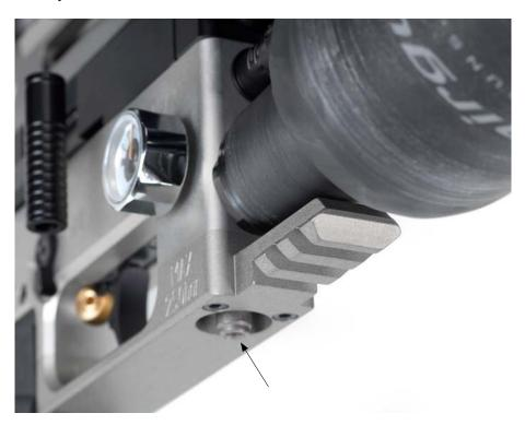
Close ventilation screw on the charging source. Charge the rifle to wanted pressure. Always check the pressure on the charging source, they have in most cases a more reliable gauge. The gauge on the rifle is more of an indicator to see if you need to charge or not. The tank pressure gauge is located on the right hand side.
